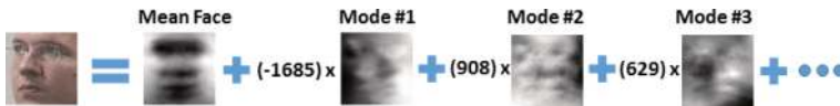
Figure 6. Representation of one face image by the mean face and first three eigenfaces obtained from PCA.
