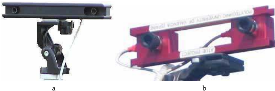
Fig. 5. Binocular stereoscopic cameras: precalibrated (a), and featuring variable baselines and interchangeable lenses (b)
