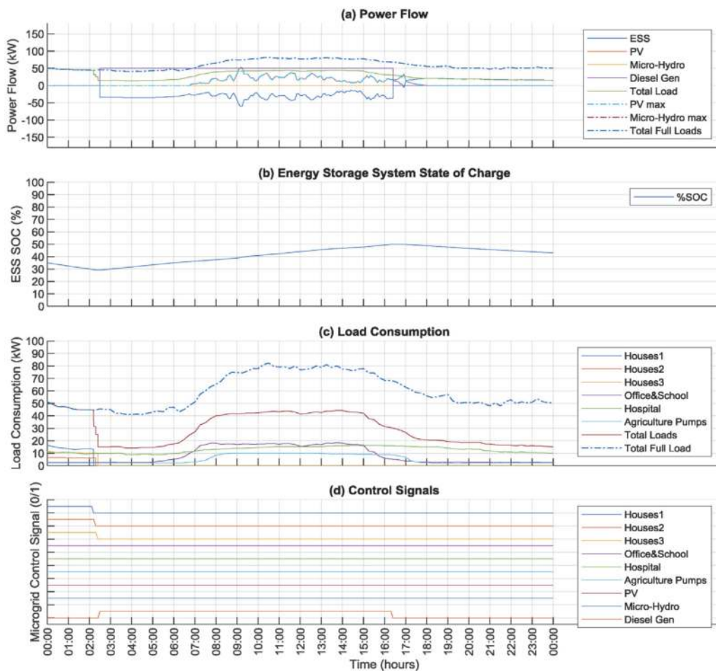
Figure 45. The simulation result for scenario 8 (a) power flow, (b) ESS SOC, (c) load consumption, (d) control signal.
