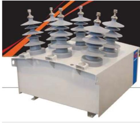
Figure 10. The REVAC recloser concept, up to 36 kV (RMS) rated maximum voltage and up to 630 A (RMS) rated continuous current [12] (courtesy of REVAC).
