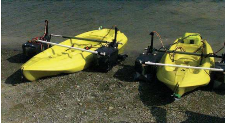
Fig. 9. Autonomous surface vehicles with propulsion systems and custom sensor and communication suites.
