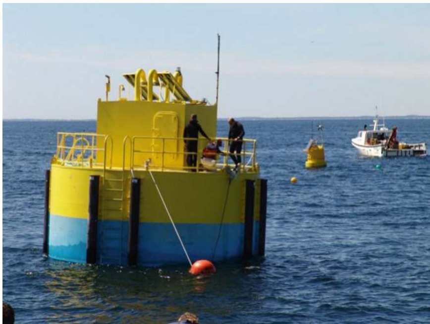
Fig. 13.10 Aquamana 20 ton feed buoy deployed at the University of New Hampshire Open Ocean Aquaculture site located 13 km offshore. The hydraulic feeder fed four submerged cages in sea conditions seas up to 10 m
