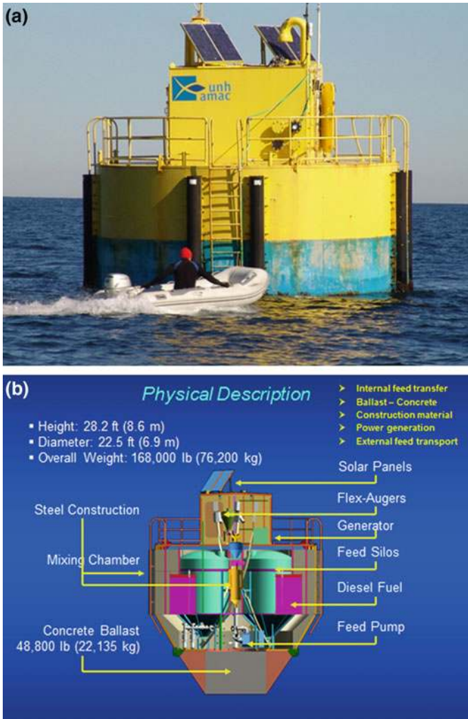
Fig. 3.8 Remote 20 ton feed buoy used to hydraulically feed four submersible sea cages up to 300 m away
