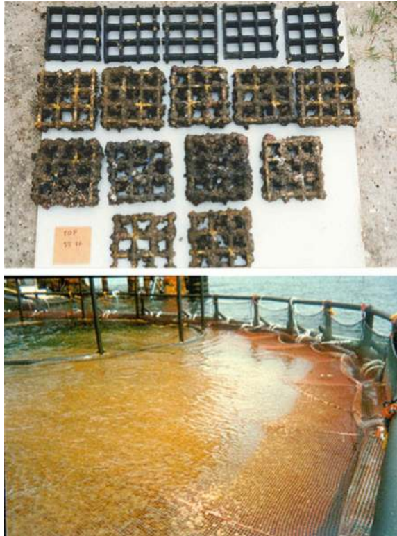
Fig. 13.4 Top Antifouling effect of copper based paint ( top row are treated samples). Bottom virtual carpet of hydroids on cage netting
