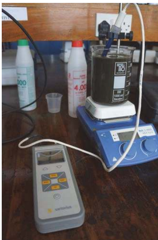
Figure 8.10 Analysis of pH for liquid faecal sludge sample. Note position of pH electrode: submerged in the well-mixed sample, but with enough clearance above the magnetic stir bar (photo: Eawag).
