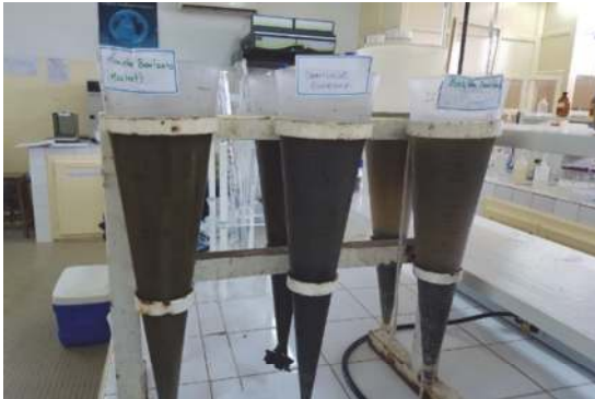
Figure 4.6 Example of an SVI settling test setup with graduated Imhoff cones (photo: Eawag).
