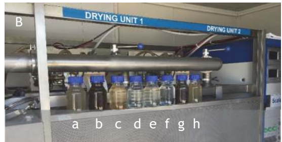
Figure 4.24 A) an experimental microwave-based faecal sludge drying unit, and B) samples taken at different points in the process: a) filtrate from the sludge press, b) concentrated sludge from the sludge press, c) ultrafiltration concentrate, d) ultrafiltration permeate, e) reverse osmosis concentrate, f) reverse osmosis permeate, g) dry sludge, and h) condensate (photo: IHE Delft).
