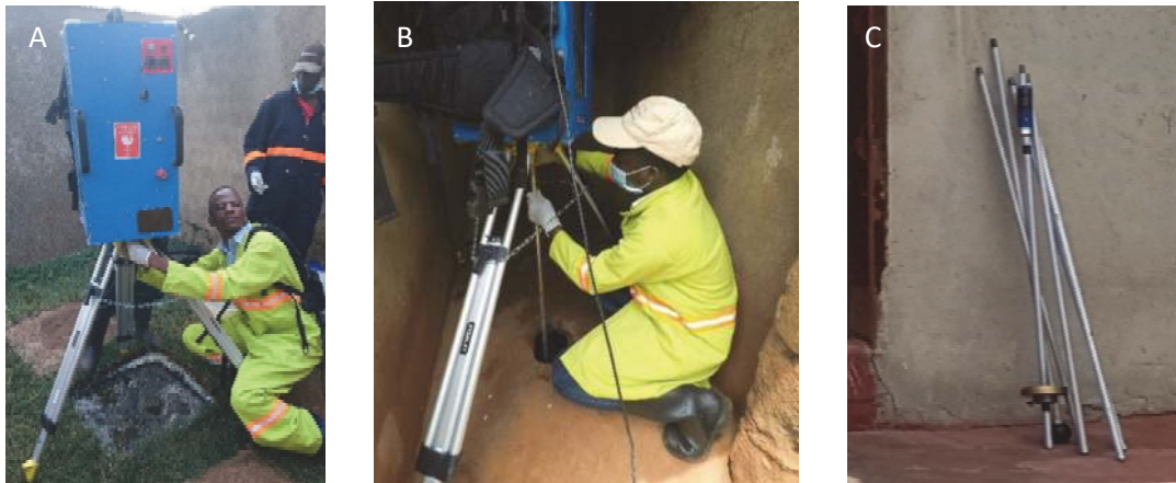
Figure 3.11 A and B) the portable penetrometer in use in Kampala, Uganda; C) the new 'P-lite' model for easier mobility in the field which is under development (photos: J. Radford).
