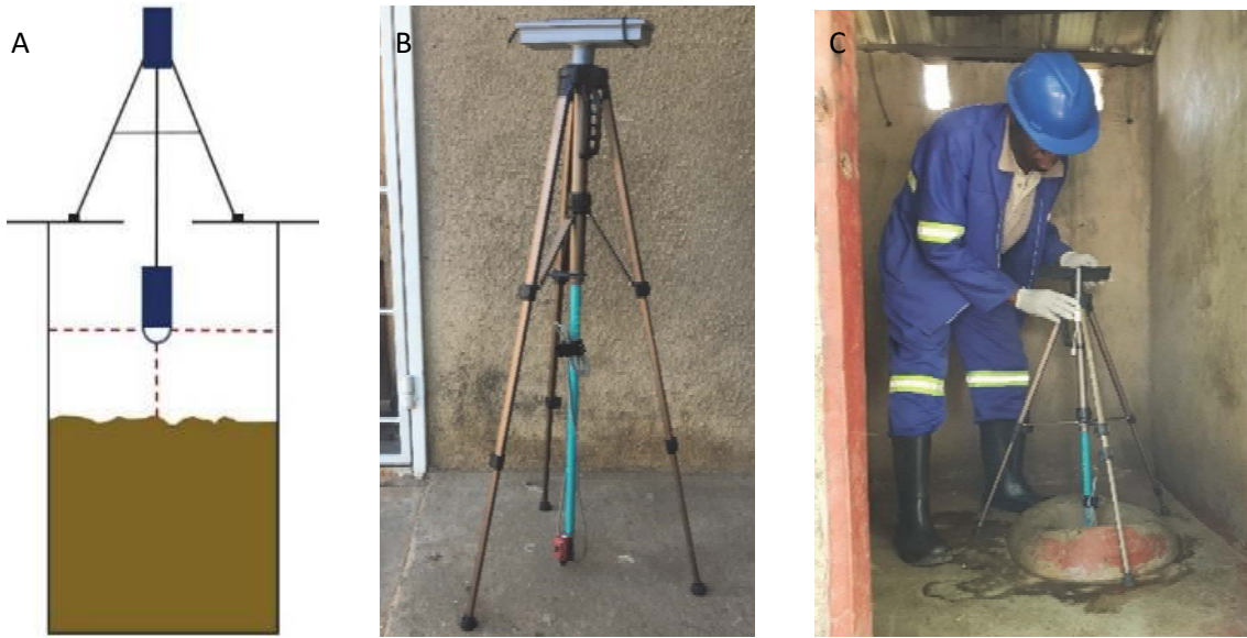
Figure 3.10 A) schematic of the Volaser with a laser measuring head that enters the containment to measure the area and distance to the sludge, with a smartphone mounted on top. Photos are from Lusaka, Zambia of (B) the prototype version used in 2019, with the Volaser placed over an access to a pit latrine (C) (photos: Eawag).
