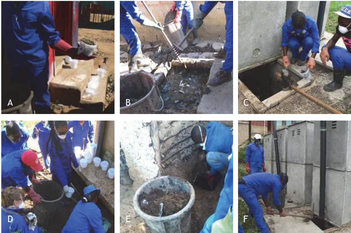
Figure 3.18 Photographs of faecal sludge samples in Case study 3.2 taken from: A) a dry ventilated improved pit latrine (VIP), B) a wet VIP, C and F) a school VIP, D) a UDDT toilet, and E) an unimproved pit latrine (photos: UKZN PRG).
