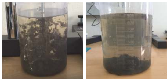
Figure 4.4 Above: steps in faecal sludge conditioning, coagulation, flocculation, and sedimentation; below left: flocculation of faecal sludge; below right: settling of faecal sludge flocs (figure: adapted from Ward and Strande, 2019, photos: IHE Delft).
