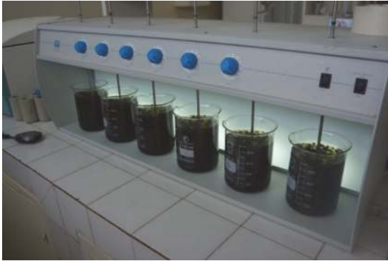
Figure 4.5 Example of a jar test setup to test suitability of a conditioner (photo: Eawag).
