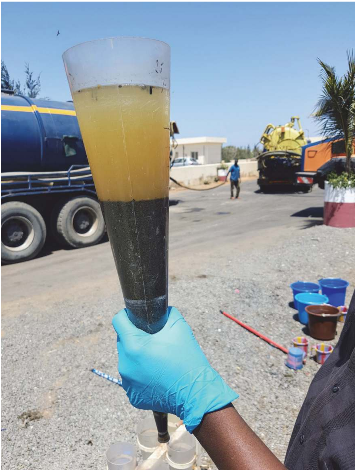
Figure 4.27 Settling tests following faecal sludge conditioning experiments at Niayes FSTP, Dakar, Senegal (photo: Eawag).
