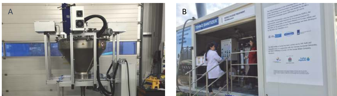
Figure 4.18 A) the bench-scale Shit Killer microwave-based technology for sludge treatment developed by IHE Delft and Fricke und Mallah Microwave Technology GmbH, and B) the follow-up prototype – the pilot-scale Tehno Sanitizer developed by IHE Delft and Tehnobirot d.o.o. (photos: IHE Delft).
