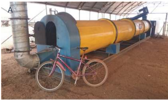
Figure 4.15 A) a rotary convection dryer operated by Pivot, in Kigali, Rwanda and B) waste cardboard is burned in a boiler and the hot gases produced are used as the heat source for drying. The sludge is pre-dried by a solar dryer before entering the convective dryer pictured here (photos: UKZN PRG).
