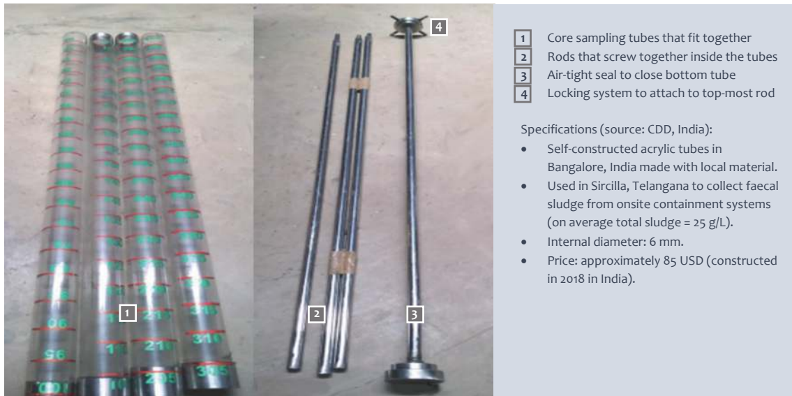
Figure 3.4 Graduated core-sampling device developed by CDD, India (Prasad et al., submitted, photos: CDD, India).
