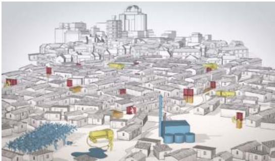
Figure 1.1 An example of the role of integrated faecal sludge management in city-wide inclusive sanitation (CWIS), with networked solutions including sewer-based and non-sewer-based sanitation solutions. Colours illustrate the faecal sludge management service chain. Red: user interface; orange (underground): onsite containment; yellow: collection and transport; green: treatment; blue: end use as resource recovery (source: Eawag).
