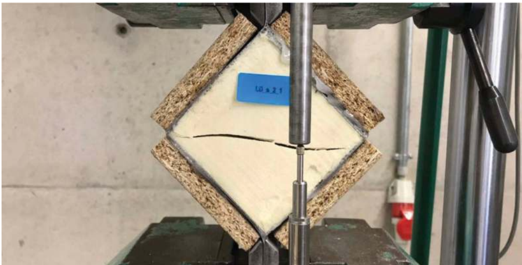
Figure 4. Plastic hinge square shear test – Shear fracture.
