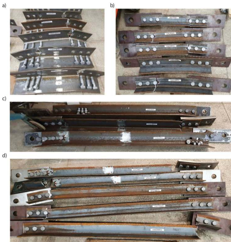
Figure 3. Overview of the specimen failure modes. a) Short L120×120×8 specimens after tests, b) Short L90×90×6 specimens after tests, c) Long L120×120×8 specimens after tests, d) Long L90×90×6 specimens after tests.
