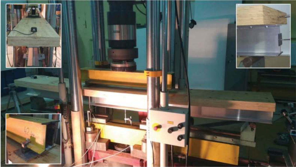
Figure 4. The aluminium-timber composite beam in the bending test (Chybiński & Polus 2019).
