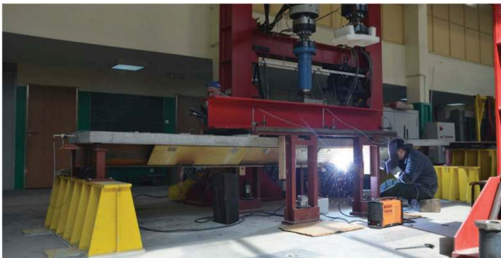
Figure 4. Welding of a strengthening plate.
