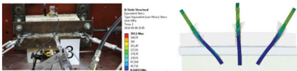
Figure 6. Failure models of three-anchor anchorages bonded at an angle of 60 degrees: experimental test and FEM model.
