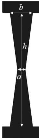
Figure 1. Butterfly-shaped link geometry with thickness ( t ).
