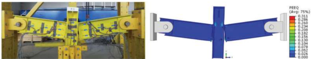
Figure 1. Comparison views of experimental and numerical test of joint with 10 mm flush end plate.
