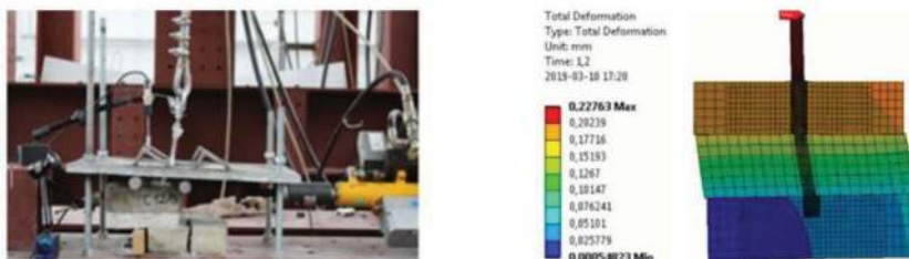
Figure 5. Failure models of 90 degree bonded anchorage: experimental test and FEM model.
