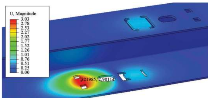
Figure 5. View of the displacement for the bottom chord of the joint WN4.
