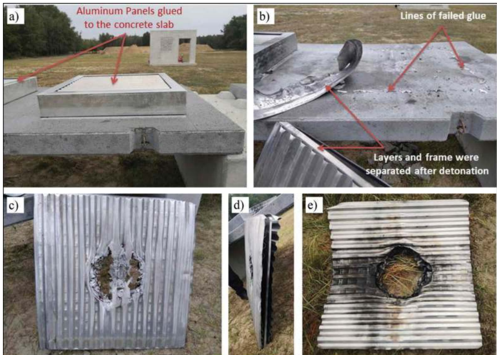
Figure 5. The failure modes of the aluminum panel after 3 rd detonation.
