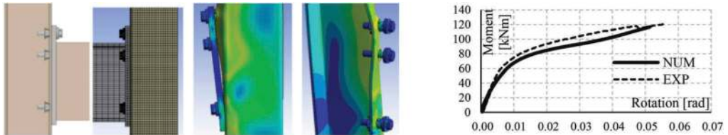
Figure 9. Caption of node and bolts' deformation – EN: T03_2 (EEP: typology B) and M-\Phi diagrams: experimental (Mesquita (2019)) versus numerical.
