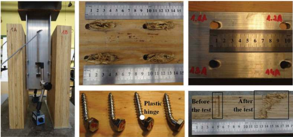
Figure 3. The push-out test specimen after the test (Chybiński & Polus 2019).
