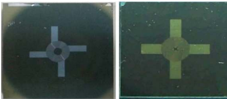
Figure 9. The prototypical photos of the substrates with metal microelectrodes and photoconductive layers for HOD.
