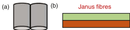
Figure 5.1 The use of side-by-side electrospinning to prepare Janus fibres. (a) The side-by-side spinneret, and (b) the resultant Janus fibres.
