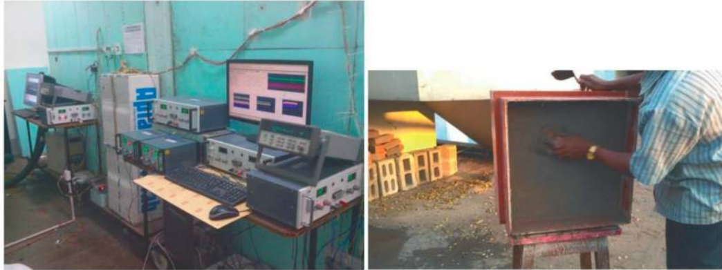
Figure 7. Guarded hot box test setup with data logging and wall panel under preparation.
