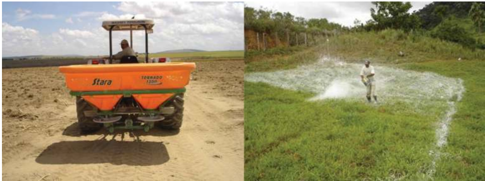
Figure 3. Equipment for the distribution of limestone in large sugarcane plantations, and a small rural producer applying limestone to previously demarcated areas.
