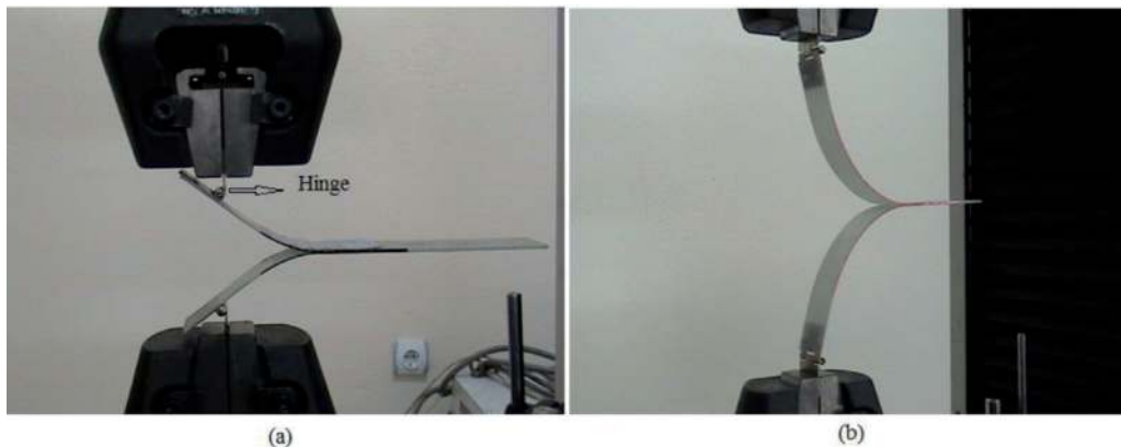
Figure 6. Overview of loading device and test setup of DCB specimen and delamination a) initially b) progress.
