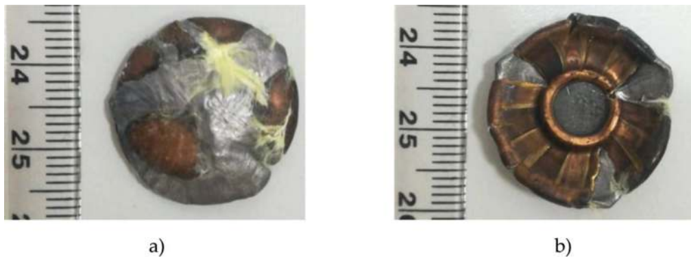
Figure 15. The bullet extracted from the sample panel presented in Figure 14. (a) Front view. (b) back view of the same bullet.
