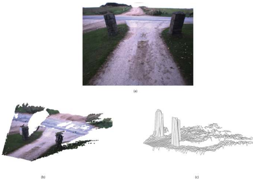
Figure 2. Example of two different space representations in which (b) is a point cloud representation, whereas (c) is the relative DEM, both geometrically describing the scene in the camera image (a).
