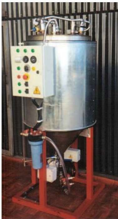
Fig. 8. Transesterification batch reactor
