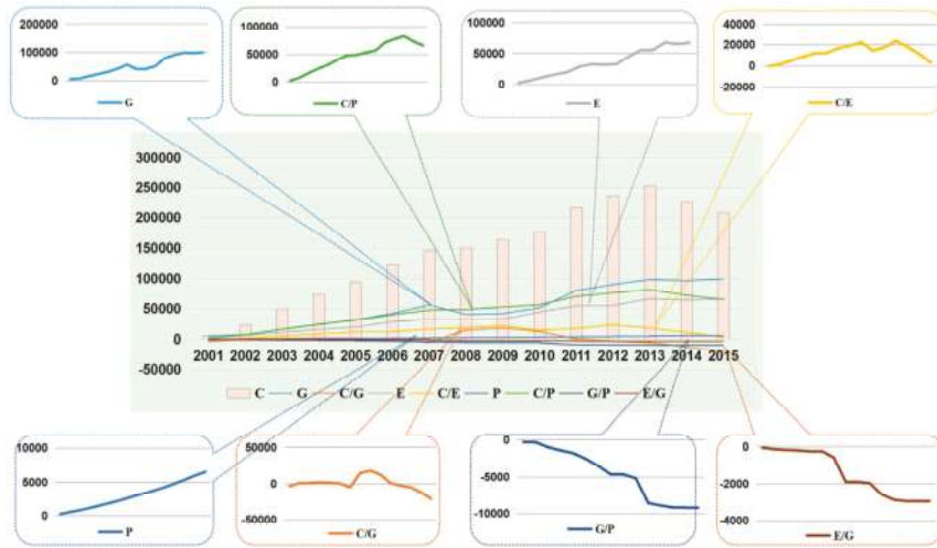
Figure 3. Cumulative contributions of various facets of the power industry to changes in carbon emissions. Unit: 10^4 tons.
