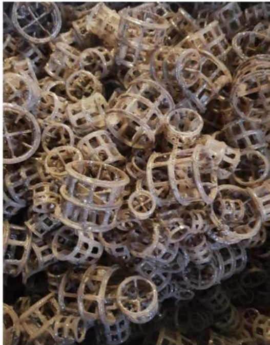
Figure 10.25 High surface area packing material used in the Nijhuis ammonia recovery system.
