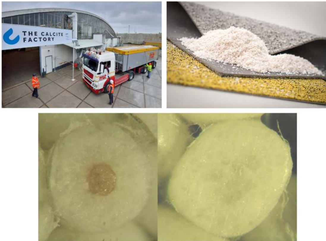
Figure 12.8 (a) The calcite factory (Amsterdam, The Netherlands); (b) Beneficial re-use of ‘Dutch Calcite’ for the production of carpets; and (c) comparison between ‘Dutch Calcite’ and conventional sand-calcite pellets.
