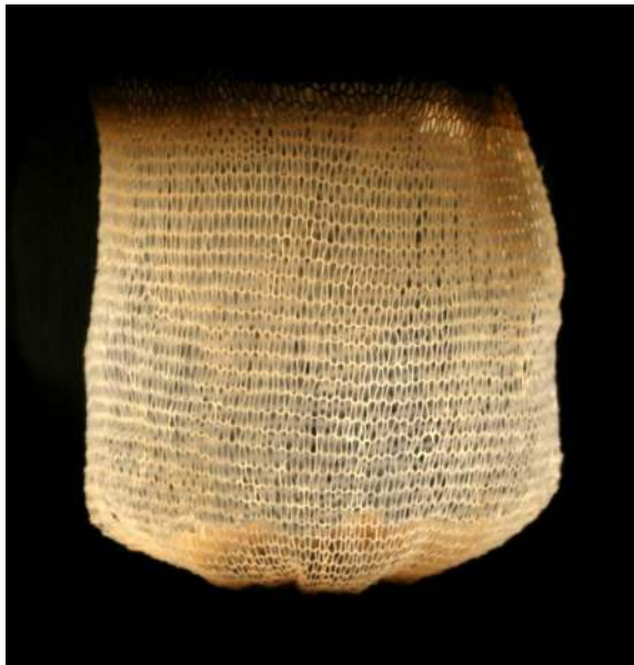
Fig. 2.4 Gas mantle burning at its highest setting. Photograph taken by Fourpointsix, August 2008. CC BY-SA 3.0, https://commons.wikimedia.org/wiki/File:Glowing_gas_mantle.jpg
