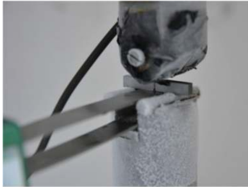
Figure 18. KLST specimens ( 4 \times 3 \times 22 \text{ mm}^3 ) from material 15CH2NMFA.
