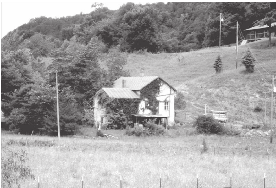
Figure 7.18 (Continued) View of the Roth house from the public road across the floodplain, 2009. The level of the floodplain appears to be close to the base of the house, suggesting aggradation of more than 10 ft (3 m) since 1874.
