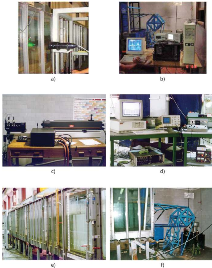
Figure 1. Experimental apparatus: (a) LDA probe; (b) DANTEC FVA signal processor and process computer; (c) laser coherent Innova and Dantec 2D fiber flow optics; (d) process computer with a AD/DA board for the wavemaker control; (e) a part of the wave channel; (f) the wavemaker.
