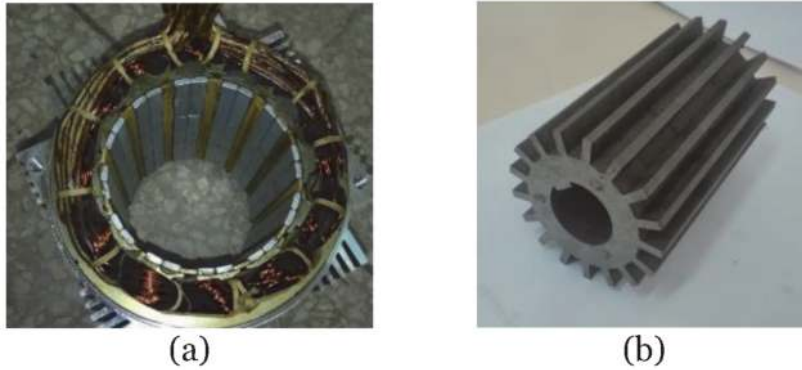
Figure 28. 12-slot/17-pole FRPMM prototype: (a) stator; (b) rotor.
