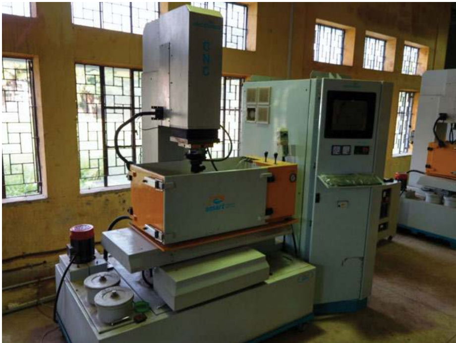
Figure 9.1: Machining setup of EDM process.
