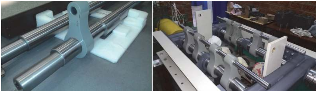
Figure 11. Connecting yokes mounted with the eccentric shafts.
