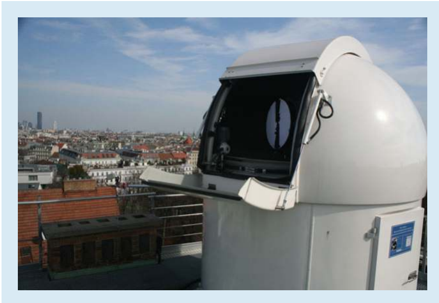
Fig. 18.19 Receiver at the Hedy Lamarr quantum communication telescope for the first free-space long-distance entanglement distribution experiment with a high-dimensional degree of freedom (Image by Mario Krenn, copyright University of Vienna)
