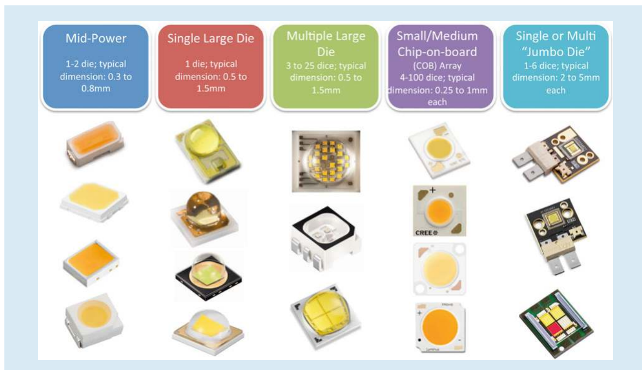
Fig. 5.17 Wide variety of solutions for high power LED packages. Images from Philips Lumileds, Osram, Cree and Luminus
