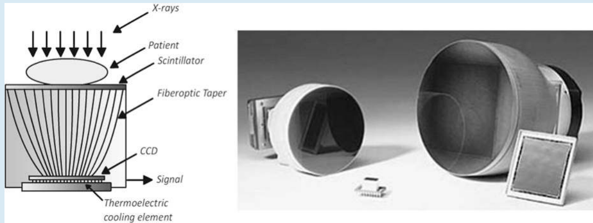
■ Fig. 13.38 In digital X-rays, a fused fiberoptic taper is used to guide the light image from a scintillator an electronic CDD detector array for processing and visualization
