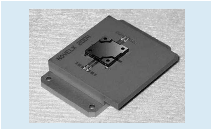
■ Fig. 6.16 A fully assembled miniature Si-wafer-based column. The dimensions of the whole column are 30 \times 30 \times 9 mm [21]
