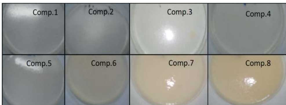
Figure 1. Comp. 1 (PVP/1wt% agar); Comp. 2 (PVP/3 wt% agar); Comp. 3 (PVP/PVAL/1 wt% agar); Comp. 4 (PVP/PVAL/3wt% agar), Comp. 5 (PVP/PVAL/chitosan/1 wt% agar), Comp. 6 (PVP/PVAL/chitosan/3wt% agar); Comp. 7 (PVP/PVAL/chitosan/PSB)/1wt% agar) and Comp. 8 (PVP/PVAL/chitosan/PSB/3 wt% agar).
