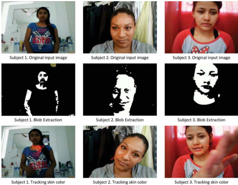
Figure 5. System of detection and tracking of the skin with the technique HS-ab. From top to bottom, the first row displays images temporarily captured by the camera, then in the second, the images can distinguish two types of blobs: black blobs (non-skin regions) and white blobs (skin regions), and the last shows the path (red color) realized by the subject.
