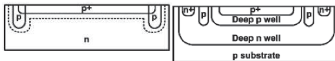
Fig. 4. Structures for avoiding PEB based on p -well guard ring at left, termination technique (2) in table 3, and deep tubs available in HV-CMOS technologies at right, termination (3) in table 3.
