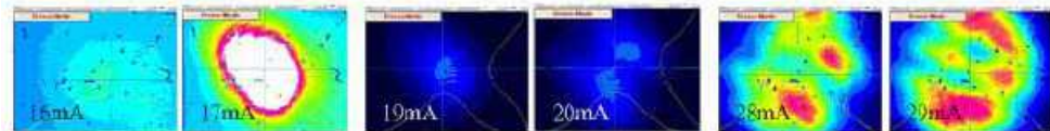
Fig. 18. The far-field pattern of 850 nm VCSEL as function of injected currents, oxidized times of 70 min
