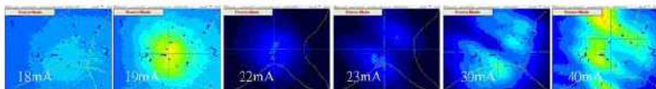
Fig. 20. The far-field pattern of 850 nm VCSEL as function of injected currents, oxidized times of 70 min
