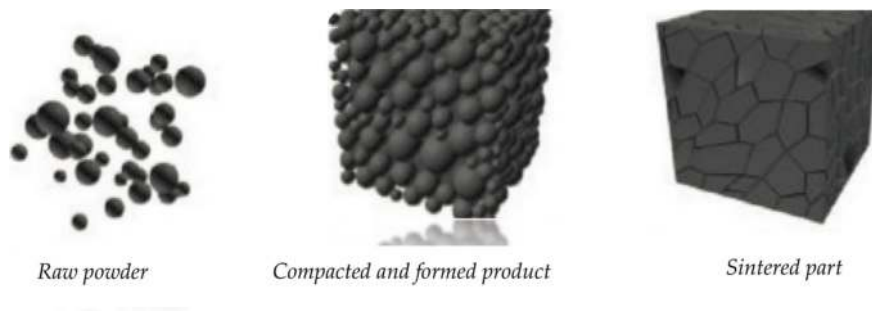
Figure 3. Powder to bonded structure during sintering.
