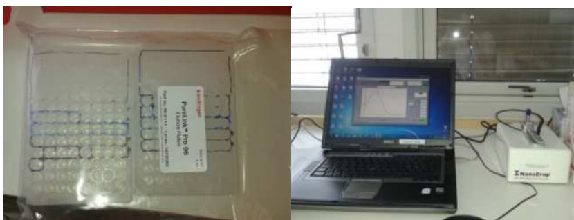
Figure 4: Left PureLink™ Pro Elution Plates with marked wells that will be used, right Nanodrop spectrophotometer connected to the computer program.
