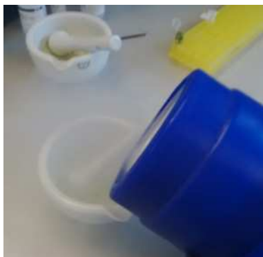
Figure 8 & 9: Grinding under liquid nitrogen.
