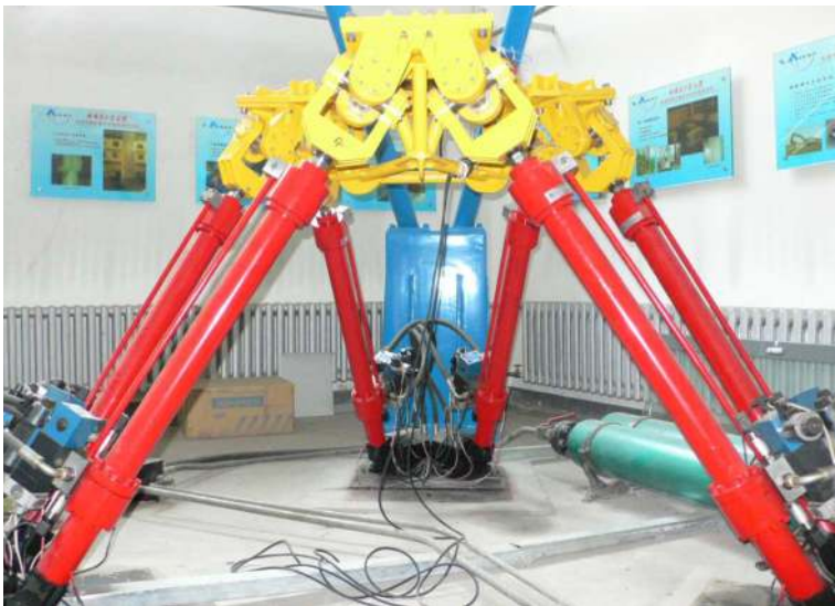
Fig. 4. Experimental hydraulic 6-DOF parallel manipulator
