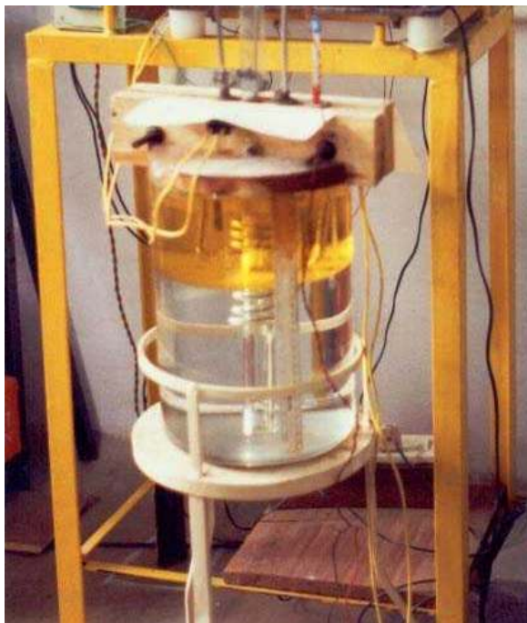
Figure 1. Transparent vertical Bridgman growth system.
