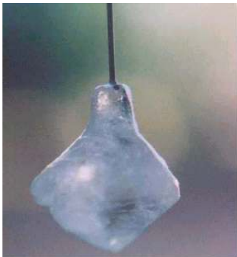
Figure 6. Grown crystal with high shoulder angle.
