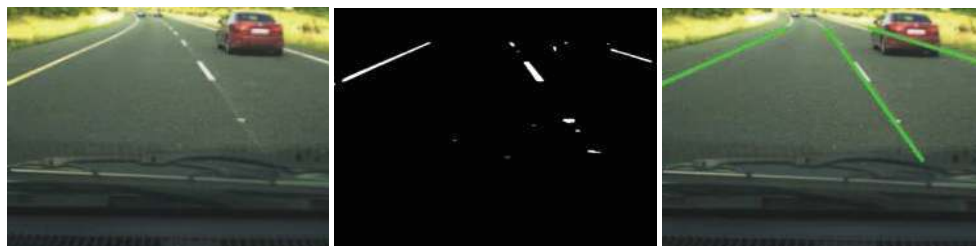
(a) Automotive image (b) Segmented roadmarkings (c) Detected lane boundaries
