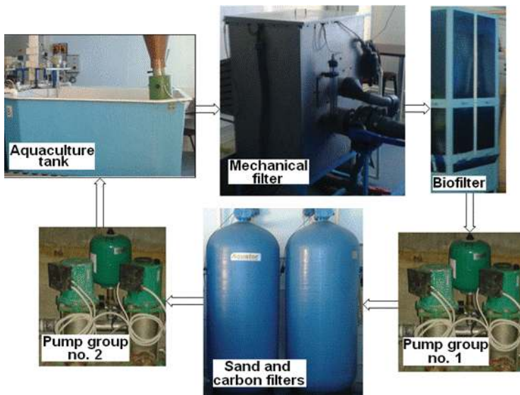
Figure 1. Structure of the technological plant.
