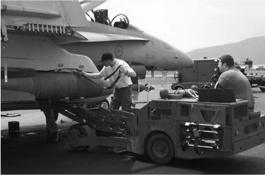
5.1. Canadian bomb loaders use an MJ loader to lift a GBU-10 Paveway 2,000-pound bomb on to a CF-18. Photo courtesy of the Department of National Defence.
