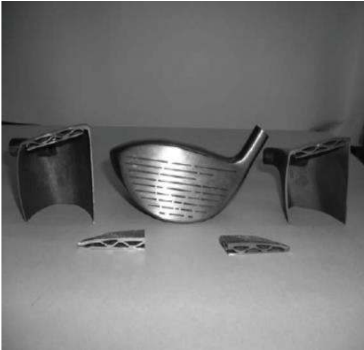
Figure 15. Components of golf club made from nanostructured Ti-6Al-4V alloy [93].
