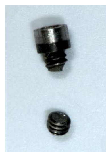
Figure 6: Fracture of a prosthetic screw
