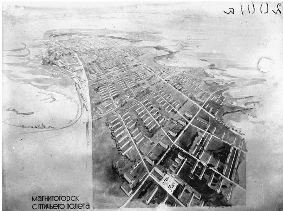
Figure 6.8. “Bird’s Eye View,” Left Bank socialist city, Magnitogorsk, Russia, 1930. Repeated rectangular blocks ( kvartaly ) for 8,000–10,000 residents extend into the distance. Planners: Tsekombank / Ernst May Brigade. MUAR, Negative VII-576.
