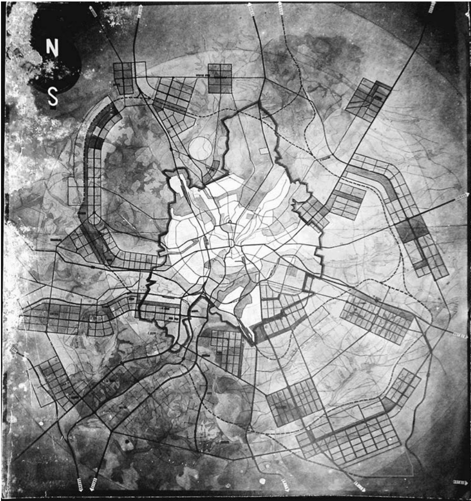
Figure 8.10. A schematic plan of linear cities. Kharkiv, Ukraine, 1929. This projective regional plan shows prerevolutionary Kharkiv in the center, encircled by a corona of linear cities, although New Kharkiv proved to be the sole built example. TsDAML M Ukrainy, f. 8, po. 1, od. zb. 264, ark. 6.
