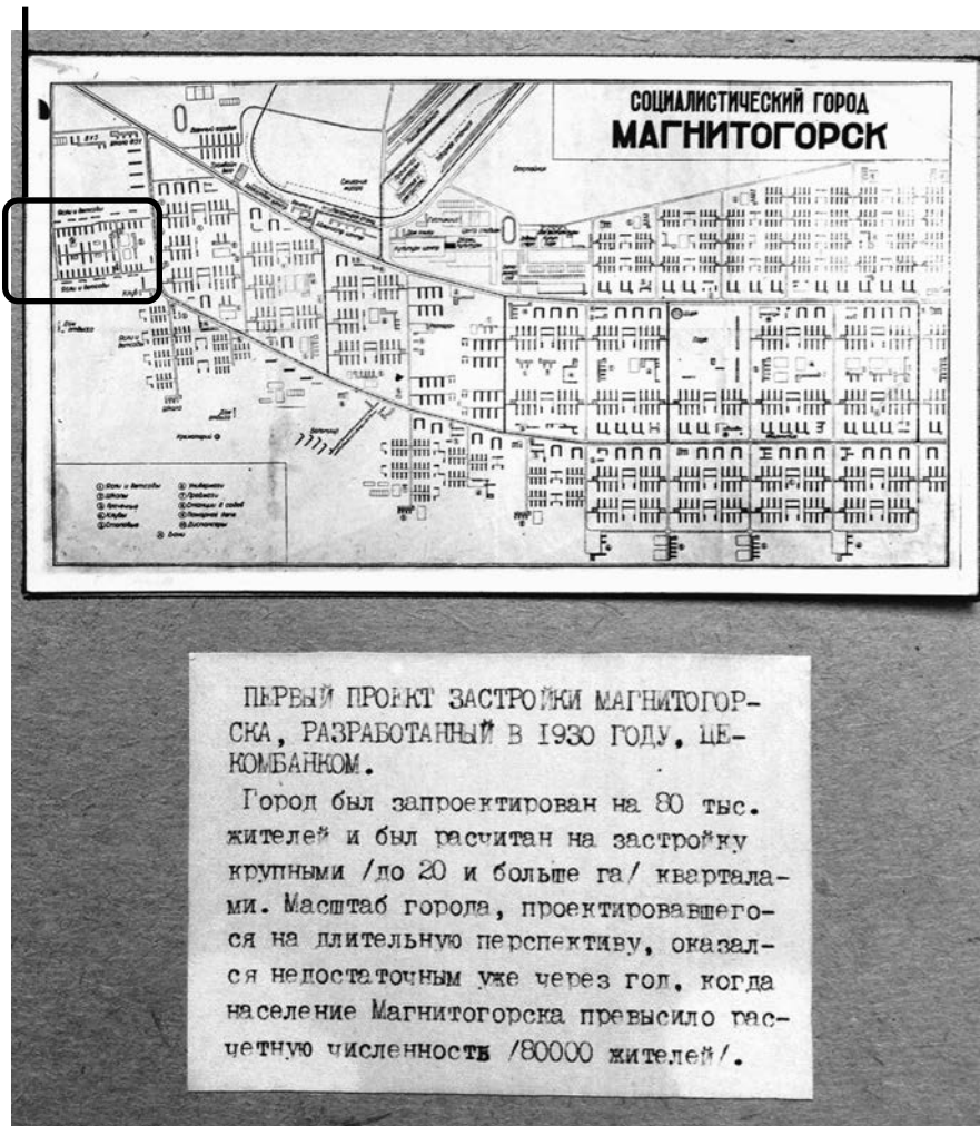
Figure 6.7. Left Bank socialist city, Magnitogorsk, Russia, 1930. The Kirov District, the only section of this scheme that was built, is located on the upper left-hand corner of the site plan. Planners: Tsekombank / Ernst May Brigade. Magnitogorskii kraevedcheskii muzei. Diagram by the author.
