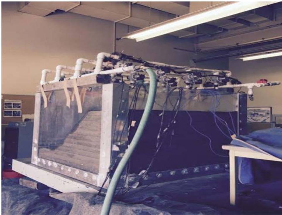
Fig. 5 Rain simulator system on slope model
