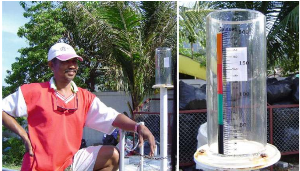
Fig. 4 Rain gauges set up in a community for observing the established thresholds
