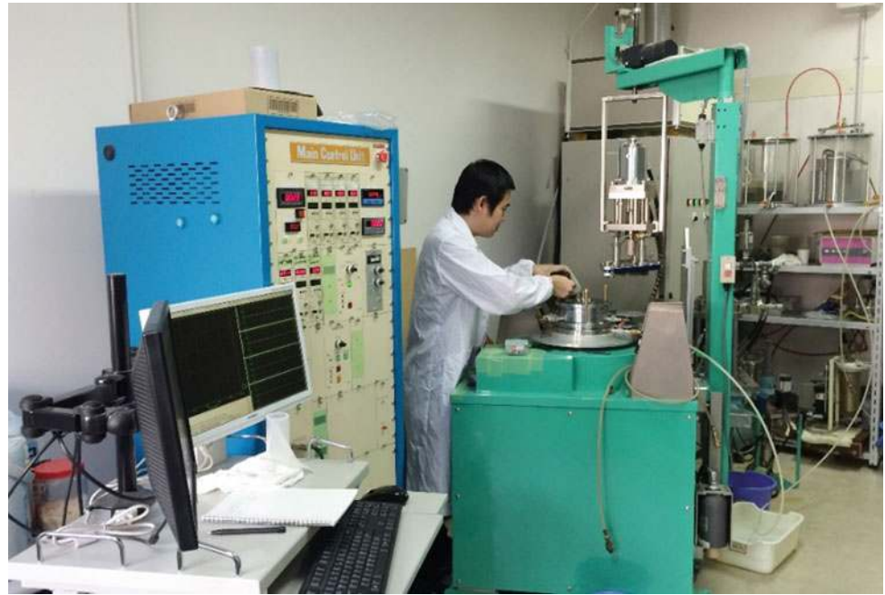
Fig. 8 ICL-2 High-stress undrained dynamic-loading ring shear apparatus (3 MPa) in the UNITWIN laboratory, Kyoto University
