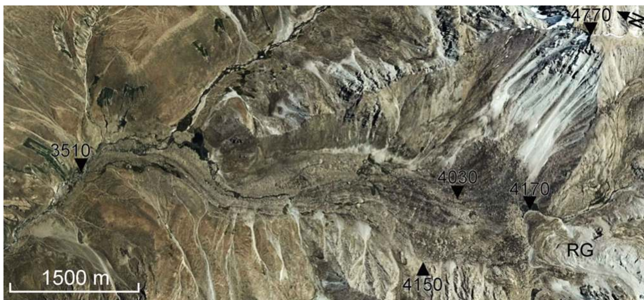
Fig. 6 The 5.5 km long Urmochdara rock avalanche in the Gunt River basin (South-western Pamir) with the striated microrelief of the deposits indicating flow-like debris motion. RG—rock glacier with a totally different morphology
