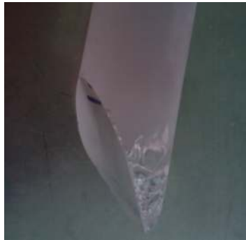
Figure 27. Cracking in the sapphire rod with stress.
