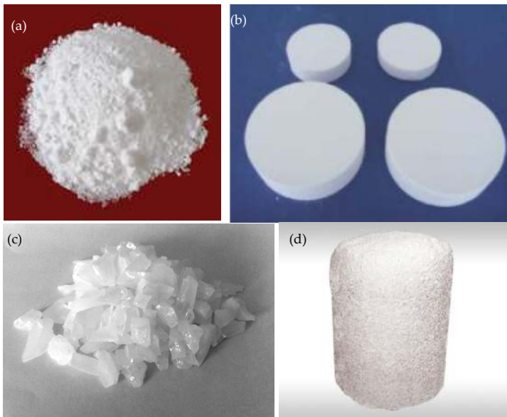
Figure 6. \text{Al}_2\text{O}_3 raw materials: (a) powder, (b) sintered charge, (c) cracked crystal, (d) polycrystalline ingot.
