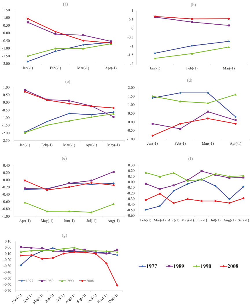
Figure A1. Plots of significant SSTs and climatic indices for forecasting Sirikit Dam inflow in January 2008 (a) Niño 3; (b) Niño 4; (c) Niño 3.4; (d) SOI; (e) Standardized SST in the South China Sea; (f) Standardized SST in the Pacific Ocean (g) Standardized SST in the Andaman sea.
