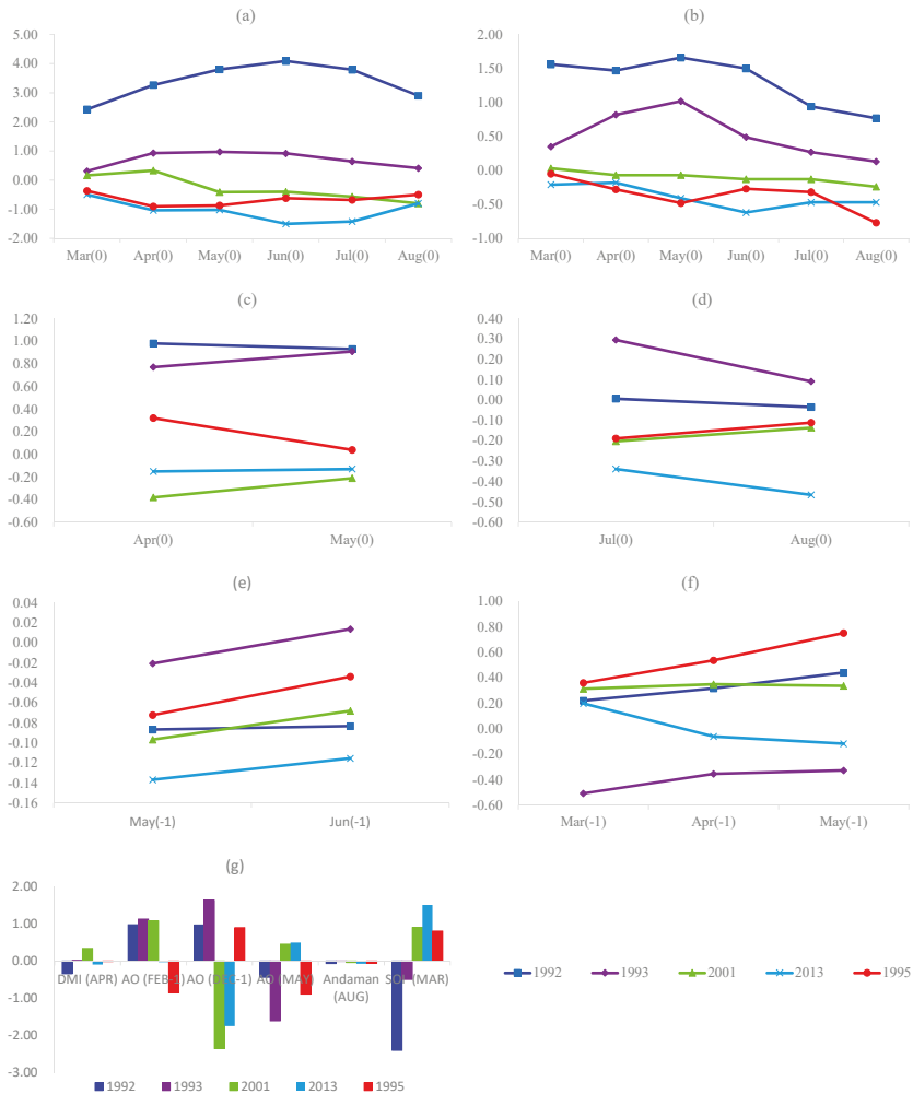
Figure A3. Plots of Significant SSTs and climatic indices for forecasting Sirikit Dam inflow in August 1995 (a) Niño 1 + 2; (b) Niño 3; (c) Niño 3.4; (d) Standardized SST in the Pacific Ocean; (e) Standardized SST in the Andaman Sea; (f) DMI; (g) Other SSTs and indices as stated in Appendix A.
