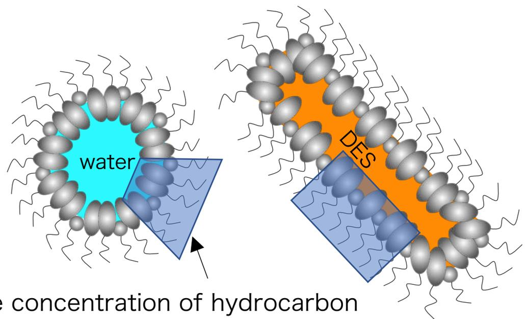
The concentration of hydrocarbon chains decreases with increasing distance from the core
