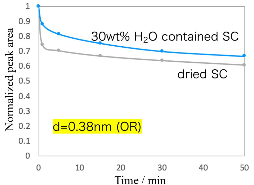
MEs disturbed hydrocarbon packing structures for both SC.
