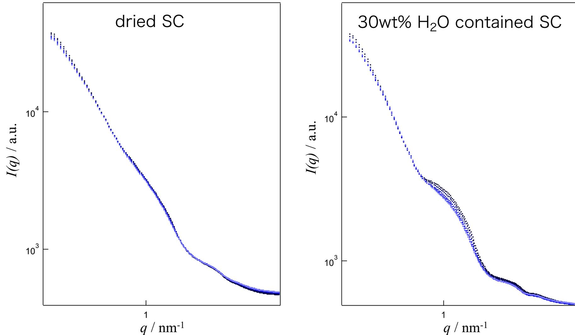
ME-DES did not disrupt the lamellar structures for the dried SC while ME-DES disrupt S-La with time for 30 wt% H<sub>2</sub>O contained SC.
