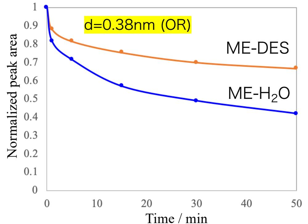
\*ME-H<sub>2</sub>O disturbed hydrocarbon packing structures more than ME-DES.
