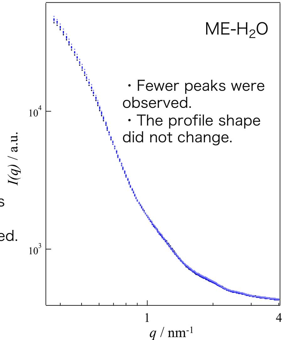
ME-H<sub>2</sub>O may strongly interact with both lamellar immediately after application of ME. After that, ME-H<sub>2</sub>O did not disrupt the lamellar structures.
