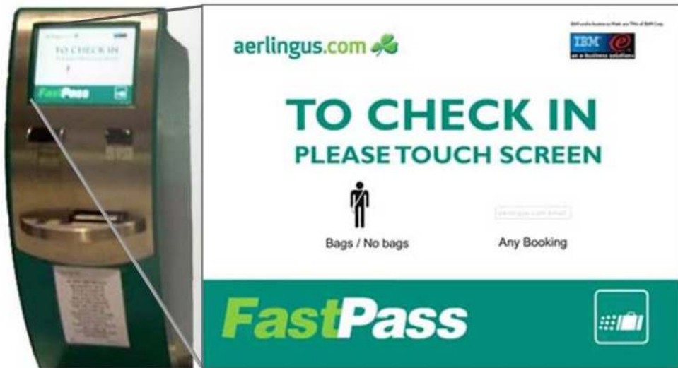
Fig. 4. Airport check-in kiosk; The interface makes use of large, short instructions and combines text labels with images for target options, supporting non-English speaking users.
