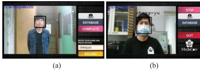
Figure 17. User interfaces for registration and face recognition. (a) Registration and setup database (b) recognition and show name.
