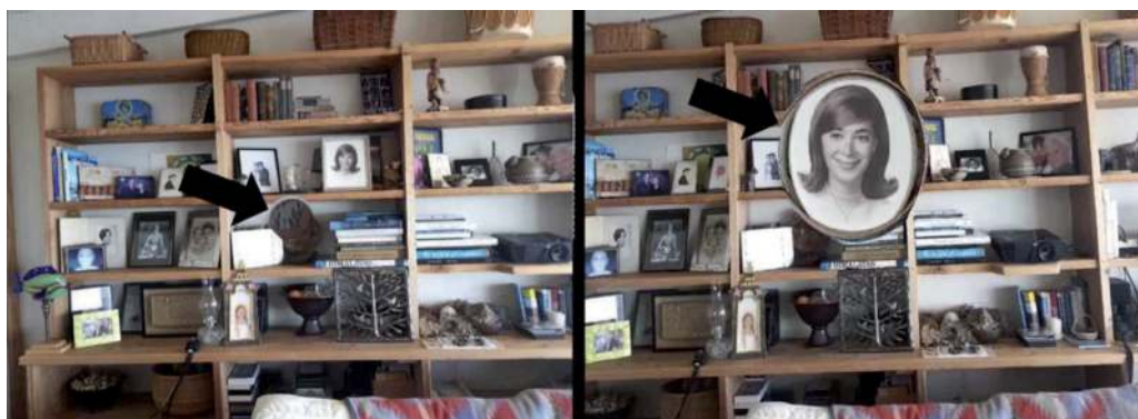
Figure 4. Example of the user-defined region or “bubble” where image can be magnified [82] (from https://tvst.arvojournals.org/article.aspx?articleid=2725386 ).
