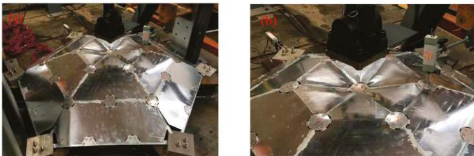
Figure 5. Failure modes of the combined lattice shell model: (a) The overall failure profile; (b) The amplified profile of a local destabilization area.
