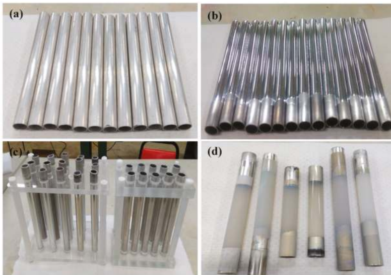
Figure 9. Batch tubular AAO process (a) 6061 Al tubes; (b) electrolytic polished 6061 Al tubes; (c) anodized 6061 Al tubes; and, (d) tubular AAO films.
