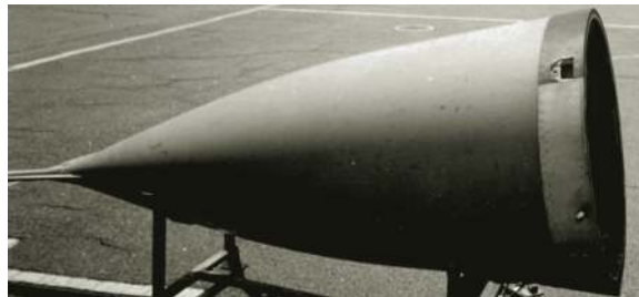
FIGURE 3.121 The nose radome of MiG-29.
