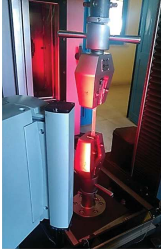
Figure 4. Tensile tester with video extensometer.
