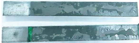
Figure 9. Failure surfaces for the DCB specimen.
